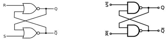
2. Build a gated S-R latch with NOR gates. Vary the inputs and observe how the enable works.
