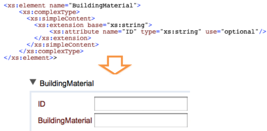
Figure 4.7: a form component transformed from a "BuildingMaterial" element
