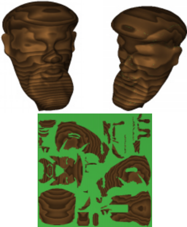
Figure 18: Head database rendered with wood solid texture (top) with (left) and without (right) overscanning, using the cube projection u -map (bottom).
