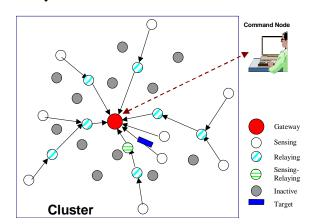
Fig. 9: A Typical Cluster in a Sensor Network
