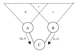
Fig. 1: The implosion problem. Node A starts by flooding its Fig. 2: The overlap problem. Two sensors cover an overlapping geographic region and C gets same copy of data form these sensors.
