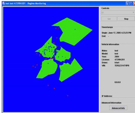
**Fig. 2** Vehicle sub-system operating regime monitoring and outlier detection module. The polygons represent safe operating regimes of vehicle subsystem.
