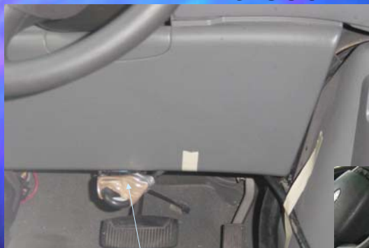
OBD-II adapter connected to a Ford Van OBD-II port
