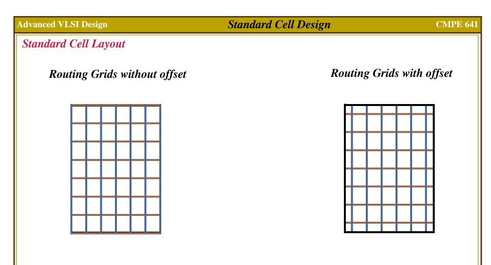
Routing grids are used by the CAD tools to route wires over the standard cells placed in the design
