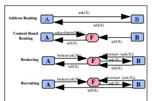
Figure 7 - Facilitators are agents that deal in knowledge about the information services and requirements of other agents. They can offer services such as forwarding, brokering, recruiting and content-based routing.
