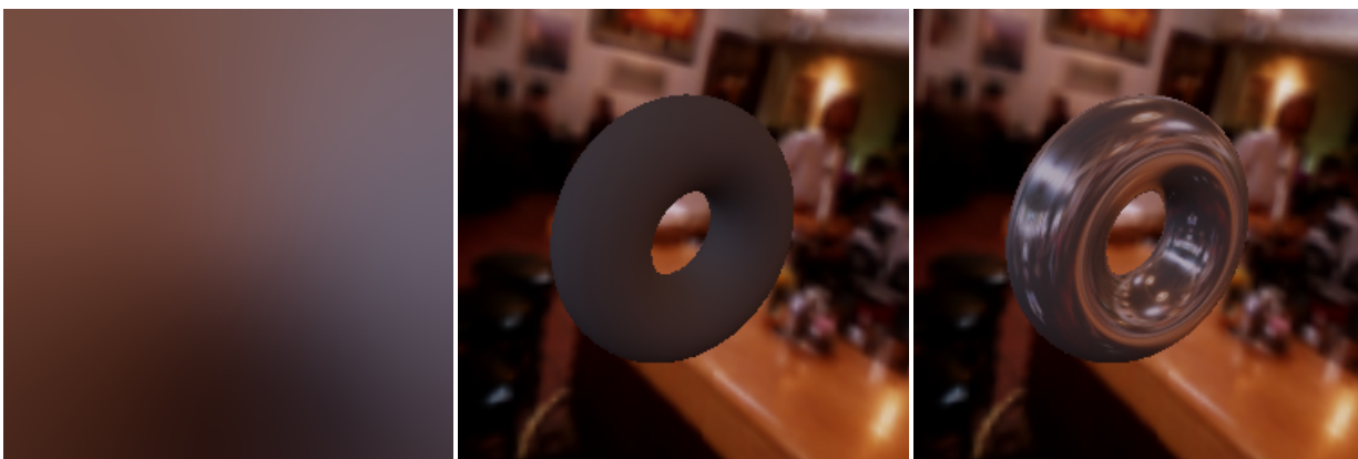
Figure 9: Left: diffusely prefiltered environment map of the cafe scene. Center: diffusely illuminated torus. Right: same torus illuminated with both a diffuse and a mirror term.
