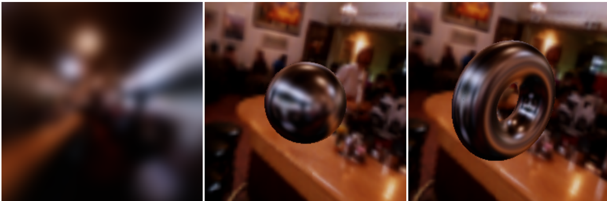
Figure 10: A prefiltered version of the map with a roughness of 0.01, and application of this map to a reflective sphere and torus.
