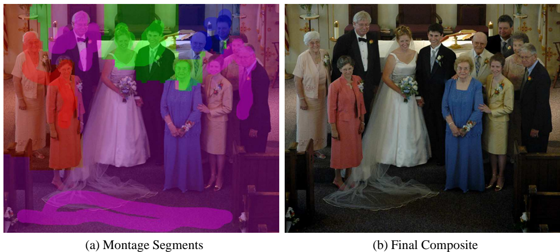
FIG. 1.2. Using Interactive Digital Photomontage segmentation and restoration to create a final composite image from multiple sub-images, where each individual color overlay indicates the sub-image that a segmented region came from (Agarwala et al. 2004)
