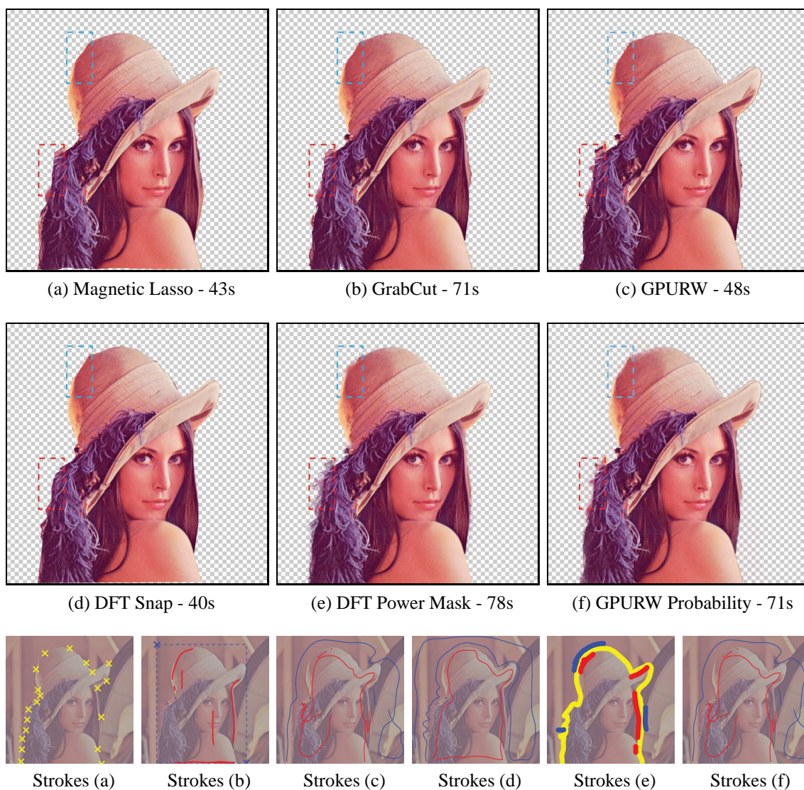
FIG. 4.9. Comparisons of different segmentation methods. Segmentations can be seen in the top two rows (the amount of time required for the segmentation in seconds is shown next to the name of the algorithm), while the inputs required to create the segmentations in their respective interface can be seen in the bottom row. Red strokes equate to foreground markings, blue to background, and yellow represent explicit-boundary indications. The boxes with dashed lines in the segmentation image are enlarged in Figure 4.10, with the blue seen on the left, and the red on the right.
