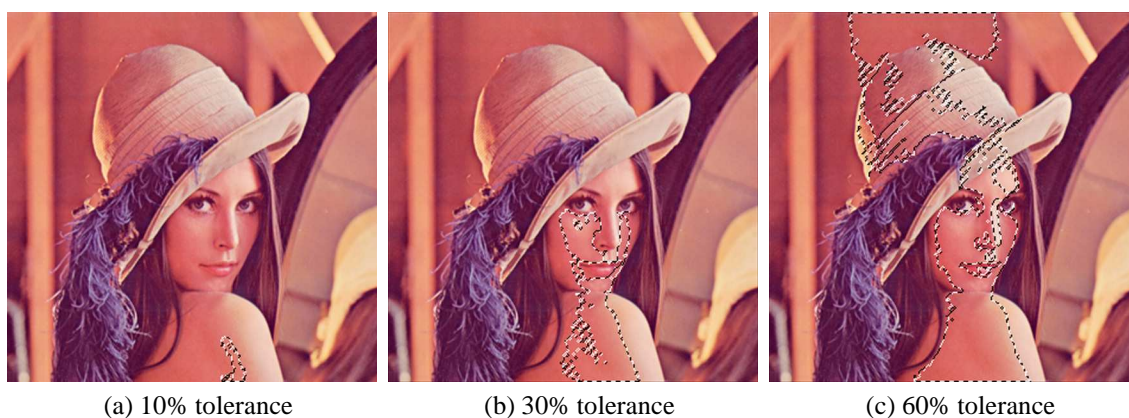
FIG. 2.1. How varying tolerance affects what is selected for segmentation using the Magic Wand tool, where the same initial pixel was specified for each selection.
